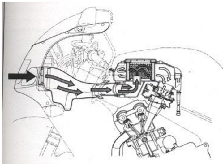
Schematic of stock ram air system on the ZX-6R
